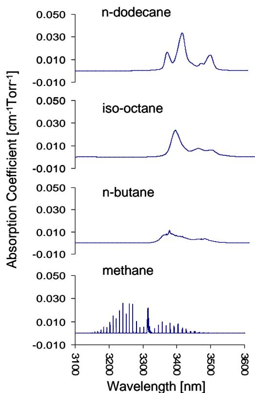
**Figure 6:** Example absorption spectra for hydrocarbon fuels.
