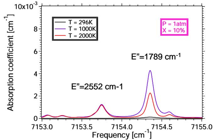
**Figure 1:** Calculated spectroscopic features for water (10%) line pair near 1.4 $\mu\text{m}$  based on HITRAN parameters.
