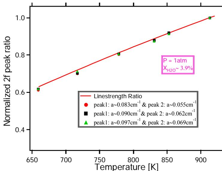
**Figure 2:** Normalized 2f peak ratio versus temperature.
