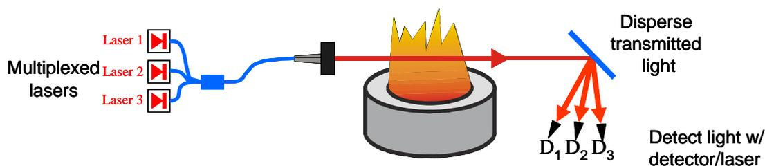
**Figure 1:** Wavelength-multiplexed absorption concept for **smart optical sensors**.
