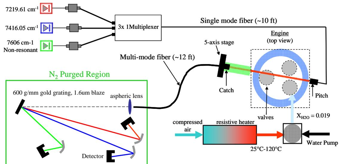
**Figure 3:** Experimental setup for the TDL absorption measurements of gas temperature inside a single-cylinder engine with optical access. Three diode lasers are wavelength-multiplexed onto a single fiber and the beam pitched across the cylinder, caught on a fiber and demultiplexed with a grating in a nitrogen purged container.
