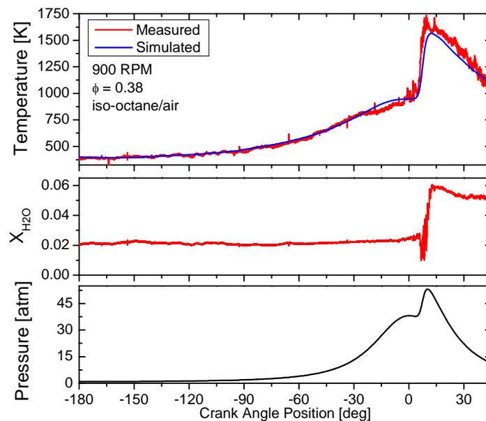
**Figure 4:** Measurements in versus crank angle for a single-cylinder engine fired via HCCI using iso-octane fuel. Top panel shows data from the TDL temperature sensor, Middle panel shows the TDL sensor data for water vapor mole fraction, Lower panel shows the measured in-cylinder pressure from a transducer.
