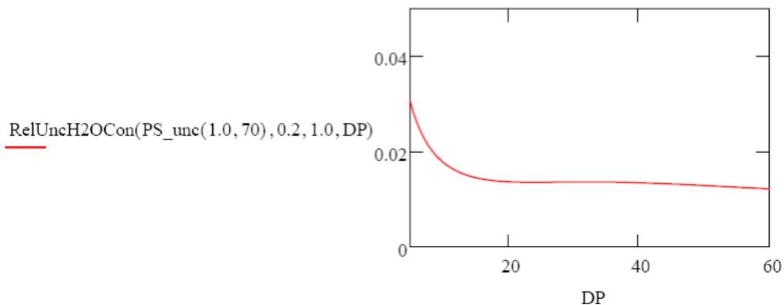
Figure 7b: Calculation of uncertainty in delivered H<sub>2</sub>O concentration as a function of measured pressure and dew point.
