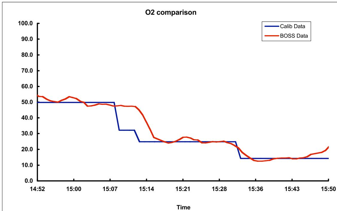
Figure 4: Zolo**BOSS** O<sub>2</sub> measurements versus calibration source under back-pass temperature conditions.
