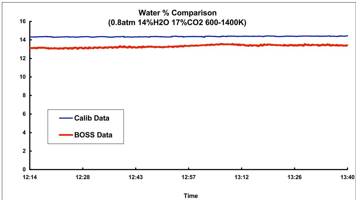
Figure 3: Water concentration validation testing over the temperature range shown in Figure 1.
