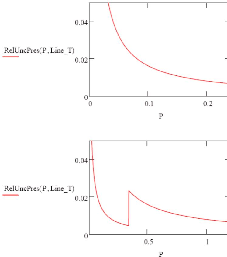
Figure 6: Relative pressure uncertainty of the pressure sensors
