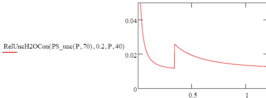
Figure 7a: Calculation of uncertainty in delivered H<sub>2</sub>O concentration as a function of measured pressure and dew point.
