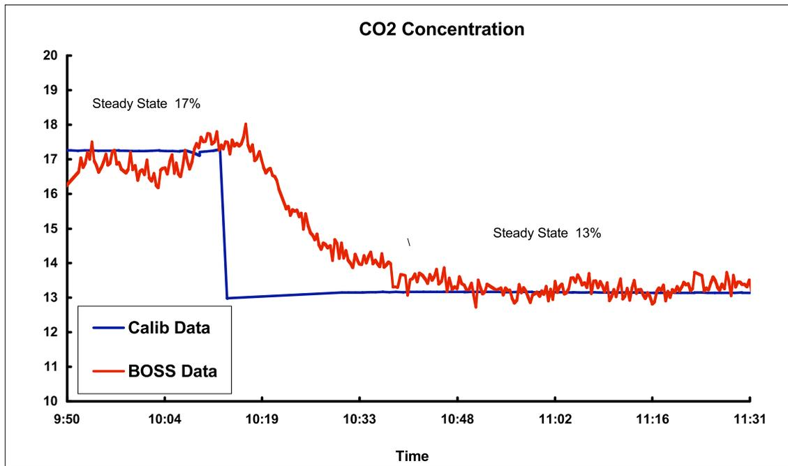
Figure 2: CO<sub>2</sub> concentration measurement validation testing. Testing was conducted at 800°F
