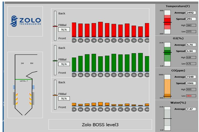
ZoloBOSS BalanceApp transforms sophisticated tomography into easy-to-read displays that can be rendered on a modern DCS. Operators use the information to see into the heart of combustion in real-time and make rapid decisions to improve performance and reduce emissions.
