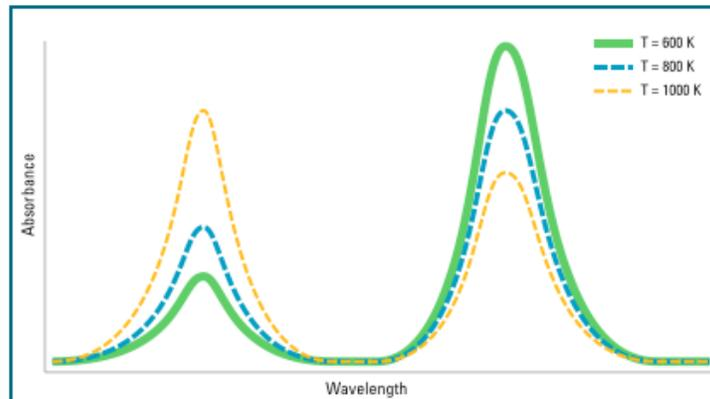
Figure 1: Schematic diagram of two absorption features that would be appropriate for temperature measurements.
