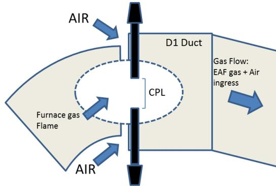
Figure 2. Location of Probes in D1 Duct
