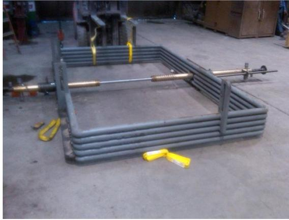
Figure 6. Probes being installed on Smoke Ring
