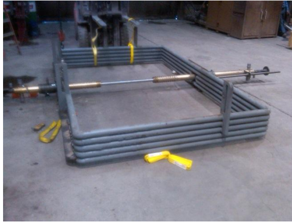
Figure 6. Probes being installed on Smoke Ring
