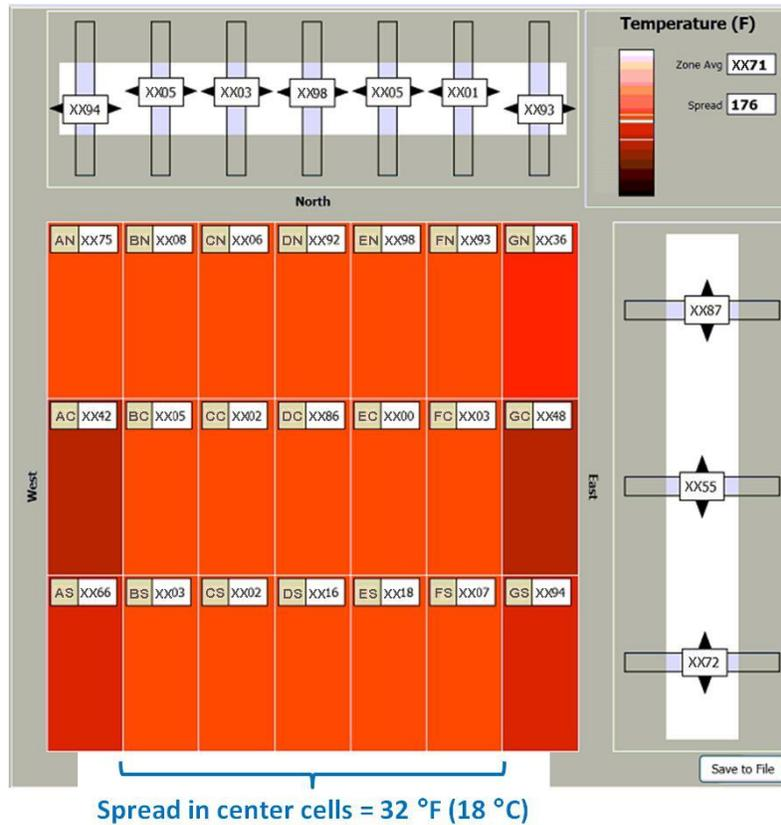
Figure 5: Improved temperature distribution after balancing Unit 1.
