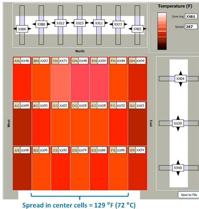
Figure 3: Example of the temperature screen of the SMR user interface. Similar screens are available for H<sub>2</sub>O, O<sub>2</sub>, and CO concentrations.
