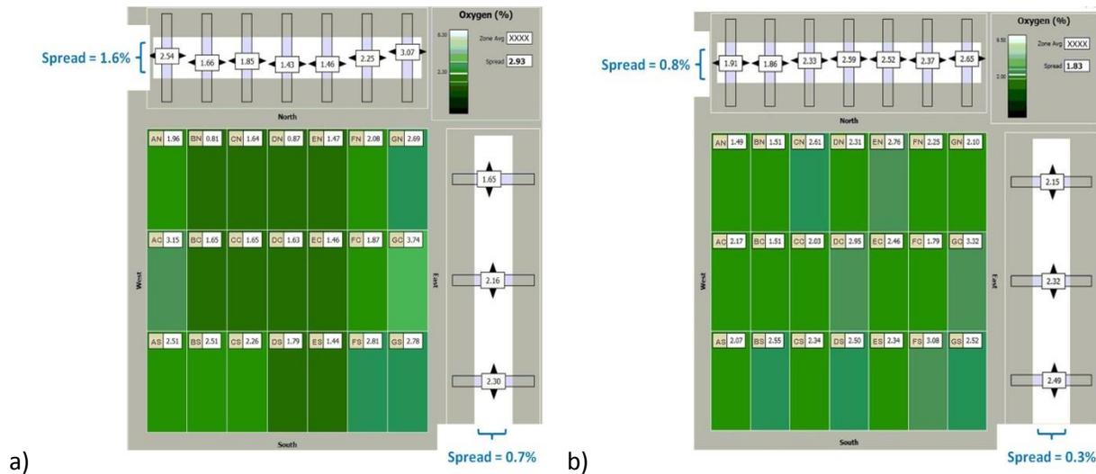
Figure 6: a) Furnace O<sub>2</sub> distribution in “as-found” state, and b) after decreasing air flow to the outer rows and balancing the fuel distribution.
